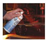
A red coloured liquid penetrant for the non-destructive testing of surfaces and structures. Many cracks in engineering materials can be deep in spite of having a very small opening on the surface, resulting in very serious or critical defects. Such cracks may be very difficult to detect by normal visual inspection and penetrant flaw detection provides an extension of the visual inspection method. The inspection is carried out using 3 products: Flaw Detector Cleaner, Flaw Detector
